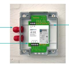
Wire into system as required (see "Wiring Configuration" on page 7). Ensure that all wiring is below the level of the front edge of the box.
