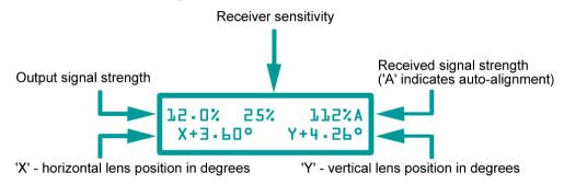
Auto alignment in 'fast' mode will take, on average, 3 minutes and in normal mode up to 30 minutes; the better the beam is aligned before auto alignment (high AQ readings) the shorter the align time. Once finished **Align Complete** will appear on the screen, simply press **left** to get back to OK and exit.
