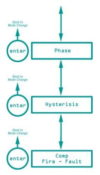
**Phase** - When using multiple beams that face each other the beam output signals could phase together and can cause unreliable readings, by setting each beam to phase differently alleviates this problem. Use the **right** and **left** keys to give each beam a different phase pattern (length between output beam sample times) you can choose between 0 (default setting) and 6. Press **enter** to return to 'Mode Change' or **down** to go to 'Hysteresis'.
