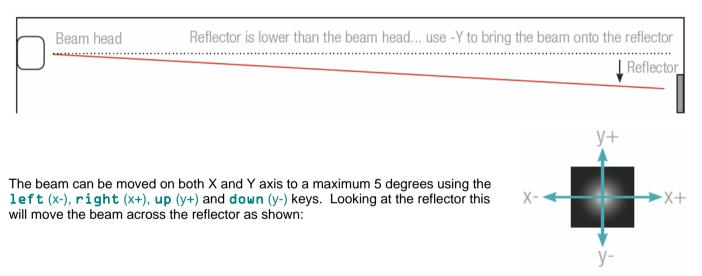
Holding the keys down will quickly scroll through to your desired position, on release of the button the screen will revert to the actual beam position and can be seen stepping toward the requested position.
